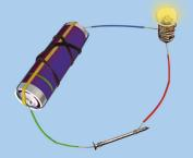
Fig. 4.2: Electric tester
